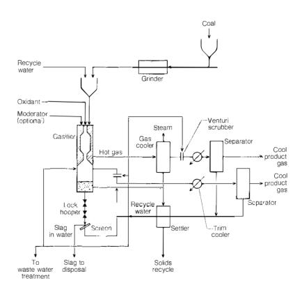
Figure 3 Process flow in the 15-t/d pilot-scale Texaco gasifier at Montebello, California.
