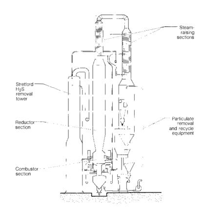
Figure 1 Combustion Engineering's two-stage atmospheric entrained gasifier. Product gases leave the gasifier, pass through the crossover duct at the top, and descend through a cooling section to the gas cleanup systems.
