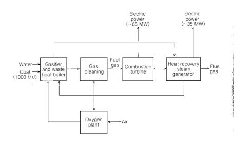
Future commercial-size plants of 500– 1000 MW will consist of multiple trains of gasifiers and combustion turbines of the same size as the demonstration plant, with economies of scale resulting from larger common facilities for coal handling, steam raising, and gas cleanup.
