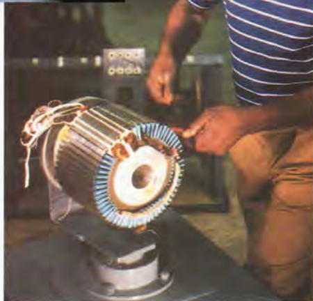
Written-Pole motors under construction
