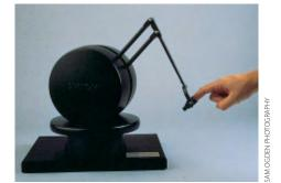
Leading scientists say computers of the future will be more like humans. Progress on this front is already under way. Shown here are a talking computer under development at AT&T and a device from SensAble Technologies called the Phantom, which uses forcefeedback technology to enable users to feel and manipulate objects in cyberspace.
