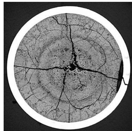
*Fuel failure is not a matter of damage to the fuel pellets themselves, but rather involves cracking of the metal cladding that surrounds them, as seen at the right in this cross-section. A crack in the cladding allows radioactive material to leak from the fuel rods into the reactor coolant.*
