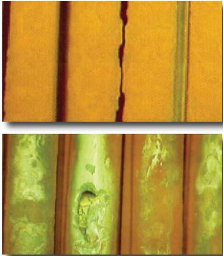
*The buildup of corrosion products, known as crud, on fuel rod exteriors (top) can distort normal heat distribution in the reactor core and accelerate corrosion and failure of the rods themselves (bottom).*
