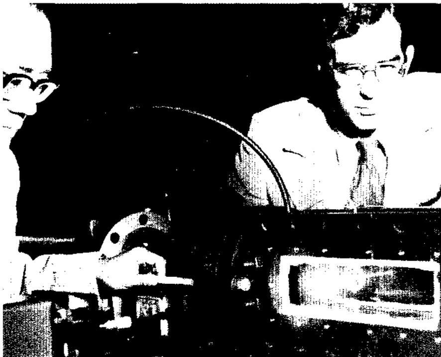
Laser beam is scattered by condensing steam in this simulation of expansion turbine conditions. Data from a range of temperatures and pressures are being used in developing more efficient turbines that are less susceptible to blade erosion by water droplets.
