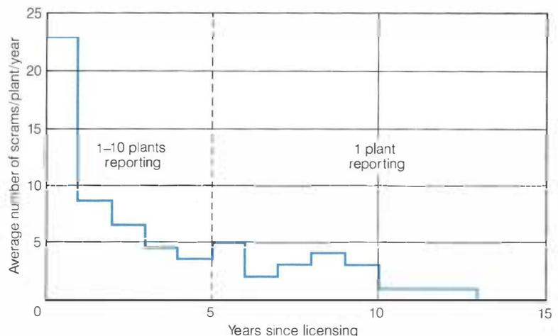
Figure 1 The learning curve with an average BWR shows sharp dependence on the length of time the plant has been in service; the number of scrams per year decreases with unit maturity.
