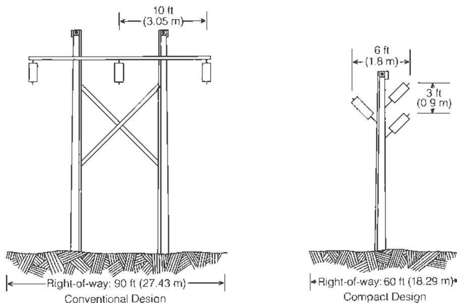
Figure 3 The advantage of compact overhead transmission line design shown should result in a significant reduction of rights-of-way needed for 138- and 230-kV lines. This should enable utilities to construct some lines at these voltage levels on city streets.
