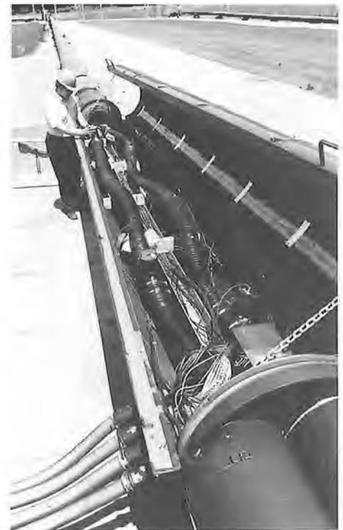
A typical test inspection port showing a solid dielectric cable splice under evaluation at Waltz Mill.
