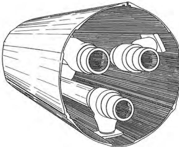
tubes required on a three-conductor system. The method of fabrication is the key to this design—three extruded aluminum segments are welded longitudinally to form the tube enclosure (Figure 2).
