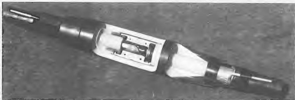
Figure 2 A novel fabrication technique (longitudinal welding) for aluminum tubes forms a reliable, rigid enclosure for this 3-in-1, gas-insulated cable rated 345 kV.
