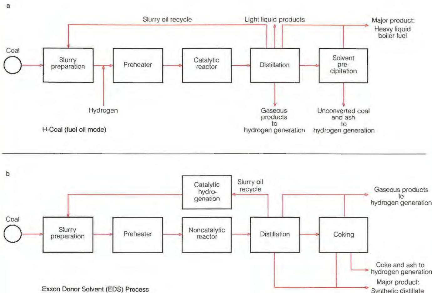
liquids having hydrogen-donating qualities. Additional cracking of these fragments and further reaction with available hydrogen results in the production of lower-boiling products. The role of gaseous hydrogen is primarily to replenish the hydrogen being released from the solvent and to quench cracked fragments, thereby preventing coke formation.
