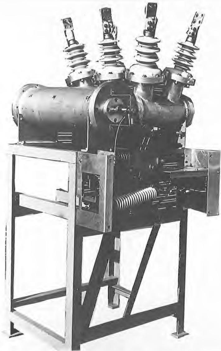
Figure 4 Laboratory model of three-phase, SF<sub>6</sub> magnetic interrupter developed under RP661 by I-T-E.
