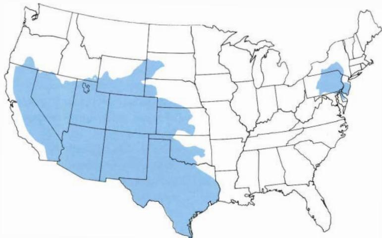
Figure 1 Projections of water availability and use indicate potentially serious water shortages in the shaded regions by the year 1990. Coupled with projected requirements for electric power generation in these regions, these estimates indicate the probable need for dry or dry-wet cooling on 14–26 GW (e) of new capacity by the year 2000.
