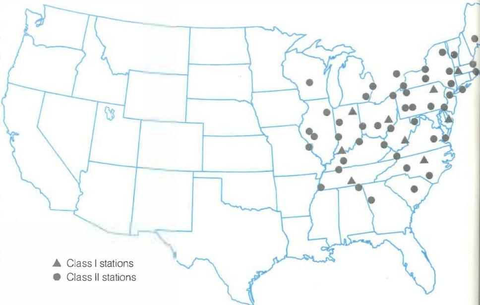
Fifty-four SURE monitoring stations carefully sited in 22 states and Canada have collected and recorded samples of ambient air from July 1977 to October 1978. Nine Class I stations operated continuously, and 45 Class II stations operated for 30-day periods during August and October 1977 and January, April, July, and October 1978.
