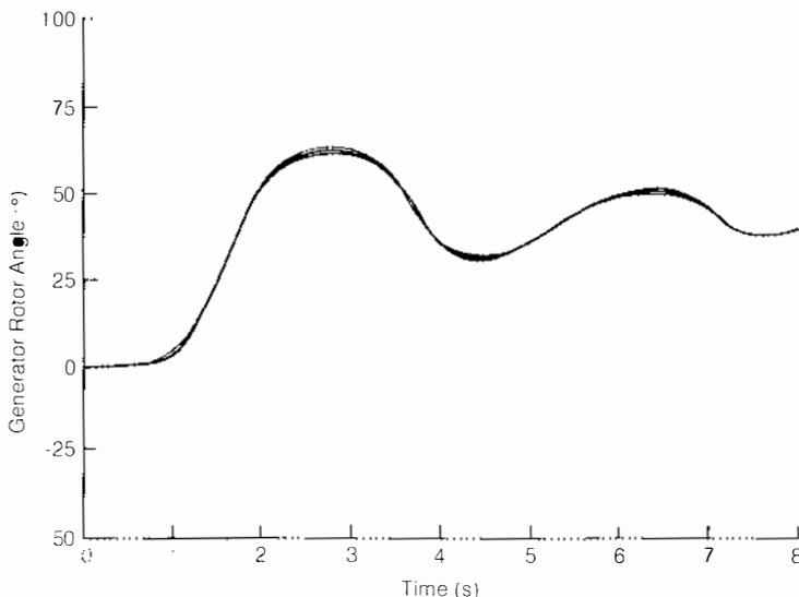
Figure 2 One of the coherent generator groups shown in Figure 1 is in the Arizona area. The coincidence of the stability swing curves for the 21 generators in this group illustrates the high degree of coherency.
