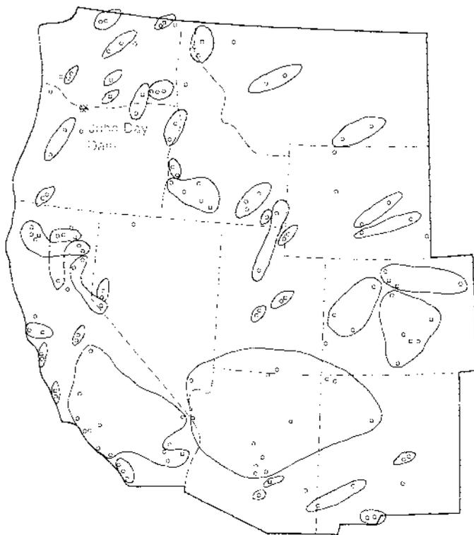
Figure 1 The geographic region of the western interconnected system. A three-phase bus fault is assumed to occur at John Day Dam on the Bonneville Power Administration system. In response to this fault, various generators in neighboring states change speed, some of them coherently (in step). These coherent groups are circled to show their geographic locations.
