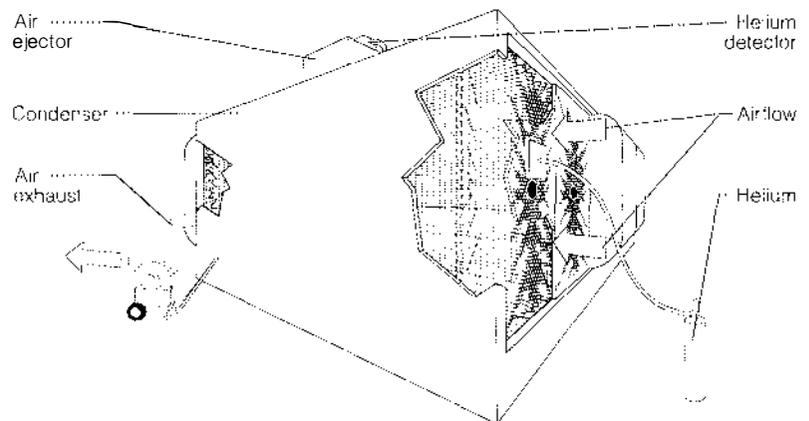
Figure 1 The tracer-gas method of leak detection in plant steam condensers.
