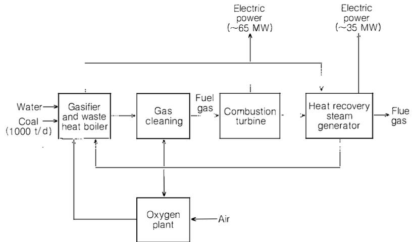
Future commercial-size plants of 500–1000 MW will consist of multiple trains of gasifiers and combustion turbines of the same size as the demonstration plant, with economies of scale resulting from larger common facilities for coal handling, steam
