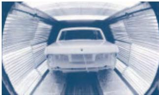
**Infrared paint curing**
