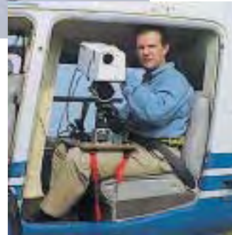
Daytime corona inspection from a helicopter is a valuable, previously unavailable capability for transmission line maintenance. In airborne field tests on the Tennessee Valley Authority system, Andrew Phillips manipulated the camera with a three-axis tripod head mounted on a lapboard that was strapped to his legs. The inspection was recorded on 8-mm videotape.
