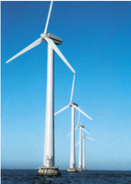
Wind power development in many parts of Europe is heading offshore both because available land is scarce and because larger turbines optimized for installation in shallow coastal areas can take advantage of the stronger winds there. These 1.65-MW Vestas V66 machines are deployed off Denmark.
