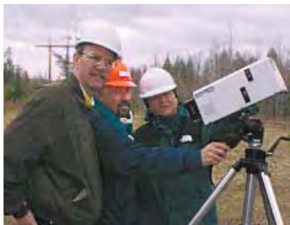
The DayCor camera was used to pinpoint corona activity on a New York Power Authority transmission line suspected of causing interference with the broadcasts of a local radio station. The results ruled out corona from the line as the cause of the interference.
