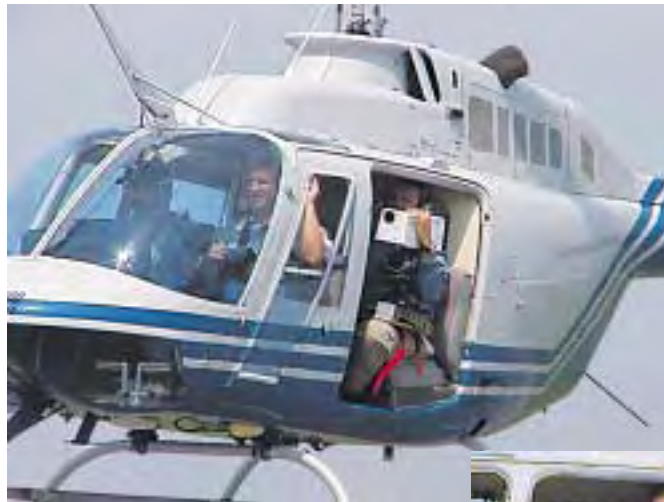
Daytime corona inspection from a helicopter is a valuable, previously unavailable capability for transmission line maintenance. In airborne field tests on the Tennessee Valley Authority system, Andrew Phillips manipulated the camera with a three-axis tripod head mounted on a lapboard that was strapped to his legs. The inspection was recorded on 8-mm videotape.
