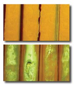
The buildup of corrosion products, known as crud, on fuel rod exteriors (top) can distort normal heat distribution in the reactor core and accelerate corrosion and failure of the rods themselves (bottom).
