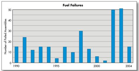
A steady increase in fuel enrichment, burnup, and operating cycles over the last 15 years has enhanced the economics of BWRs. But these operating changes, along with modifications to the water chemistry environment, have also led to an increase in fuel failures. PWRs have experienced similar problems.
