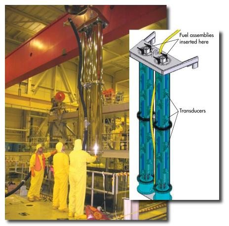
An EPRI-patented fuel cleaning technology allows utilities to remove crud from fuel assemblies during a routine reload outage. In this process, a complete assembly is placed in each of two canisters, which contain high-energy ultrasonic transducers that loosen the crud by the repeated formation and collapse of tiny bubbles. The technology, which received the prestigious R&D 100 Award in 2005, will have been applied at a dozen nuclear plants worldwide by the end of the year.
