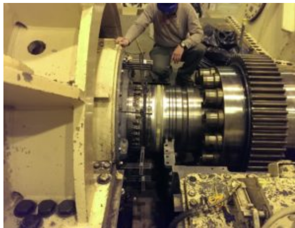
The EPRI-Suprock torsional monitoring system: The thin yellow strip on this turbine shaft is an epoxy-infused fabric that keeps electrical devices bonded in place when the shaft is spinning. Sensors and antennas are concealed under this strip.
