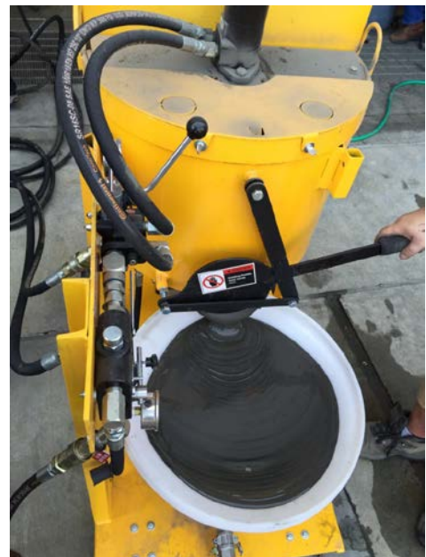
A mobile mixer used for creating paste on-site for field-scale testing.
