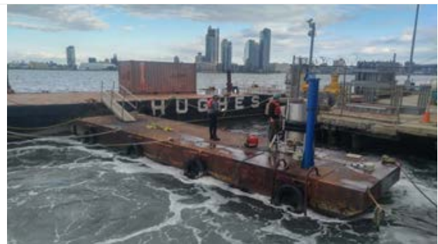
Located on a barge near Con Edison’s East River Plant, this equipment collects fish and shellfish eggs and larvae that are entrained in the plant’s cooling system and exposed to physical and thermal stress. The silver cylindrical device is lowered into the water to collect aquatic life that exit the plant.
