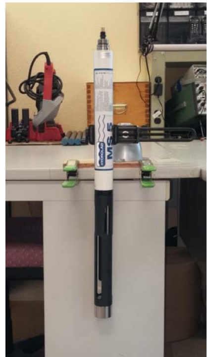
A microsensor for groundwater monitoring.
