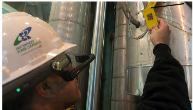
As part of an EPRI pilot study in 2018, an operator at East Kentucky Power Cooperative uses the head-mounted micro-display to scan a QR code on a valve, confirming that he is looking at the correct component. Photo courtesy of East Kentucky Power Cooperative.
