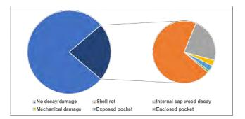
EPRI used an NLP algorithm to extract the type of decay and damage from 485,000 wood pole inspection records.
