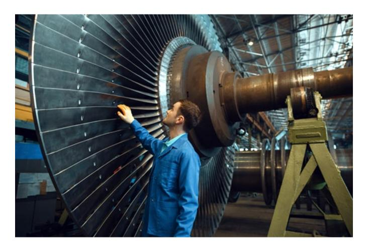
Here's how PCRT works: A technician uses a piezoelectric transducer to feed energy into turbine blades, causing them to resonate at specific frequencies. With the use of algorithms and advanced pattern recognition software, these resonant frequencies are compared with a database of frequency data to identify potential abnormalities. Based on this analysis, turbine blades with standard resonant frequencies earn a passing grade, while those with irregular frequencies fail.
