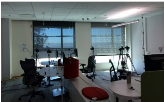
This photo inside FLEXLAB shows testing of technologies for a new Genentech office building, including automated roller shades, dimmable LEDs, and sensors to measure glare, light levels, and energy flows. Genentech staff occupied the space for a period to assess its quality under various weather conditions. Photo courtesy of Lawrence Berkeley National Laboratory.
