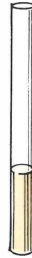
8. This waste-bearing glass occupies one-third of a canister 10 feet by 1 foot, which is transported to...
