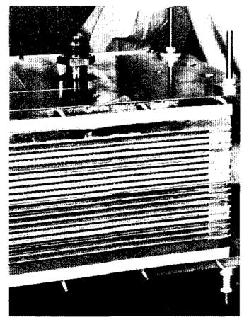
Molten carbonate fuel cell stack (20 cells) has 3-kW output and operates at  $1100^{\circ}$ F without supplemental heating, demonstrating ability to scale up from laboratory cells to hardware size (1 ft<sup>2</sup>). A 40-kW demonstration (4-ft<sup>2</sup> area) is planned in 1978.
