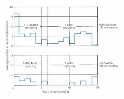
numbers should be closer to 2.5/yr with a range of 0–5 for BWRs. Figure 2 shows that PWRs exhibit the same sharp fall in scram initiators per year as BWRs, but here we have to discriminate between scram initiators involving loss of feedwater and no loss of feedwater. The former have a long-term expected average of about 1/yr, while the latter have an average of about 4/yr and the ranges are about 0-2 and 0-8.
