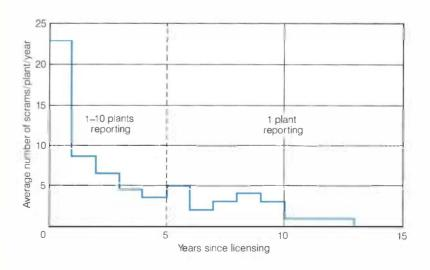
Figure 1 The learning curve with an average BWR shows sharp dependence on the length of time the plant has been in service; the number of scrams per year decreases with unit maturity.
