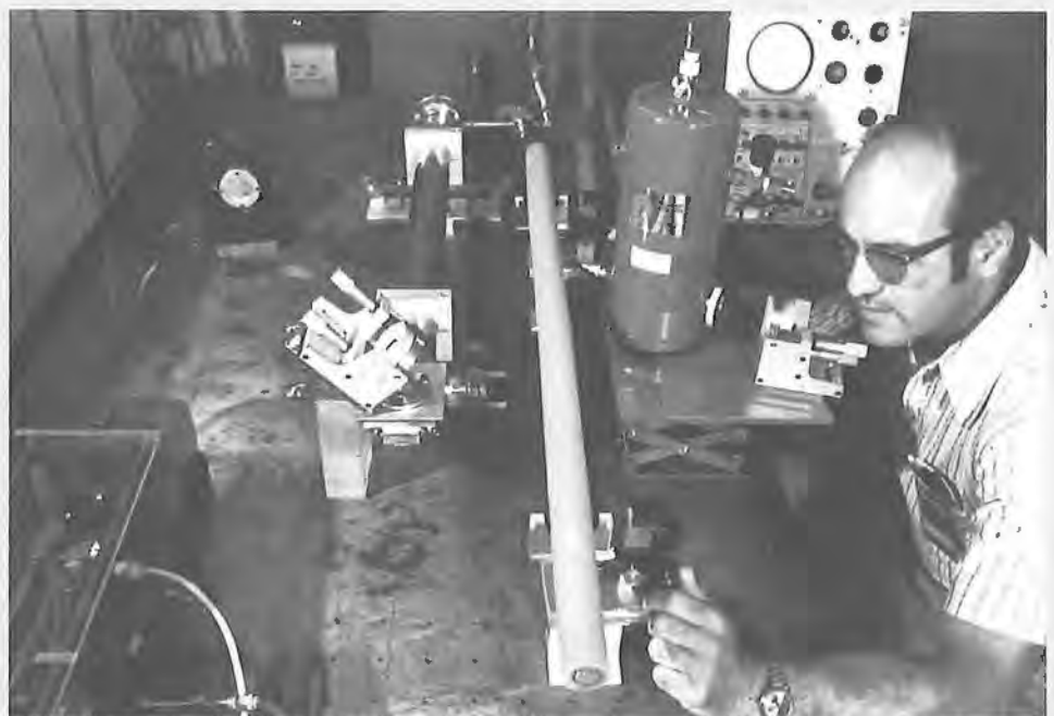
Figure 1 Laser beam detectors in the far-infrared spectrum are under development to reveal voids and contaminants in solid dielectric insulation.
