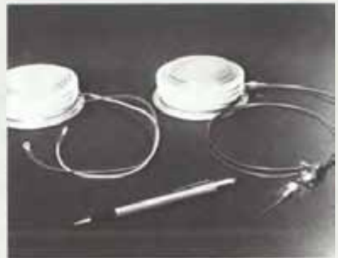
Figure 3 Comparison between a conventional Westinghouse thyristor that has electric gate control (left) and a new thyristor that uses fiber optics for gate control.
