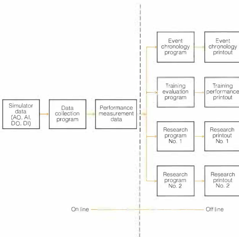
Figure 1 The structure and operation of the performance measurement system. Four types of data input and output are received by the data collection program and stored on magnetic tape. The data can then be compiled in a number of ways by different computer programs and printed out.
