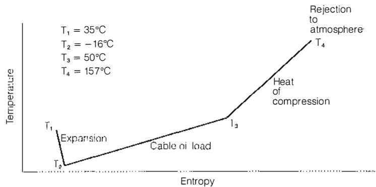
Figure 4 Entropy curve of an open-cycle refrigeration unit shows its ability to intake air at a relatively high ambient temperature (35°C; 97°F) and to expand the air to a very low refrigeration temperature for maximum cooling effect.
