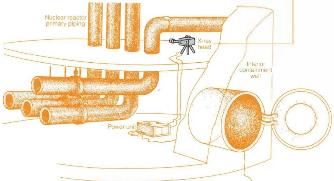
A portable radiography system for in-service examination in a power plant. The heart of the system is a small X-ray head. The measurements indicate the target for the prototype.
