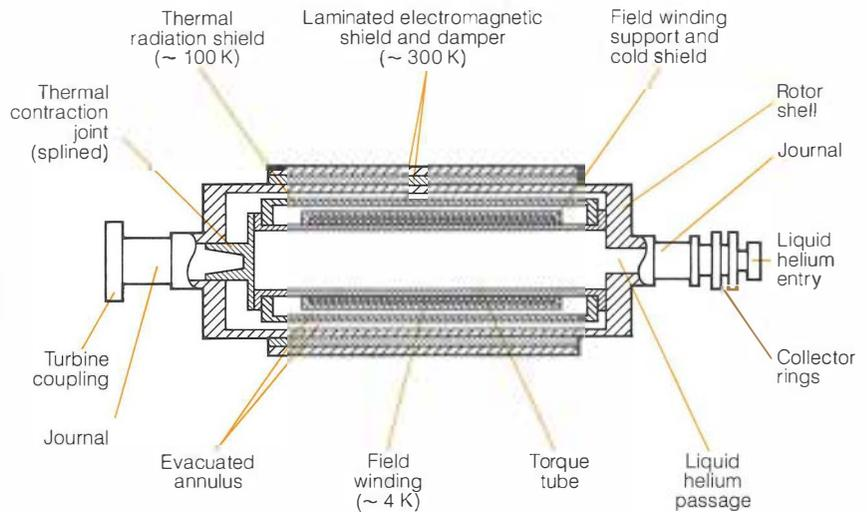
machine—its ability to withstand transient disturbances—is affected by both the subtransient and transient reactances, as well as by the rotor inertia. Despite the lower rotor inertia of a superconducting machine, which detracts from stability, transient and subtransient reactances can be reduced sufficiently to yield a net improvement.
