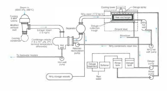
The economics of the system are closely tied to the performance of the condenserreboiler and the dry tower. Extensive fouling of surfaces in either component would be detrimental. Operating experience is the only means of determining the extent of fouling, which must be allowed for in the design. With respect to deluge cooling, the extrapolation from accelerated laboratory studies of water chemistry to long-term performance under actual on-site conditions is uncertain.
