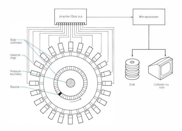
Figure 5 Conceptual layout of a gamma scanning densitometer system. A rotating radioactive source transmits gamma rays through the container and fluid to a circular array of detectors. The microprocessor is used for high-speed data storage and density profile reconstruction.
