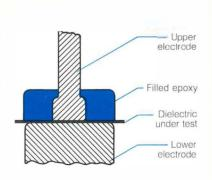
Figure 1 Dielectric test cell employed by Institut de Recherche de l'Hydro-Quebec to measure insulation breakdown strength as a function of temperature.
