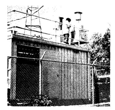
SURE Class I monitoring station in Philo, Ohio. The device on the roof resembling a stovepipe collects respirable-size particles from the atmosphere on filters, which are replaced every three hours throughout the day. The metal building contains gas monitors, calibrators, pumps, and telemetering equipment for data storage and transmission via telephone lines to ERT laboratories for analysis.
