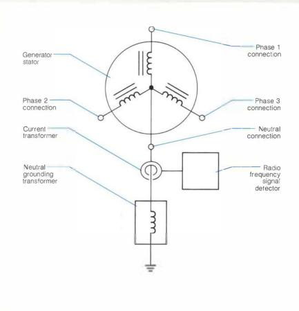
in two of these generators by subsequent disassembly and visual inspection, performed at the request of the station managers. In one case, arcing was discovered on a loose copper cover plate (Figure 7). The cover plate was replaced and the unit was returned to service. The RF signal spectra from before and after the repair are shown in Figure 9. The signal levels after the repair were typical of those encountered with nonarcing generators.
