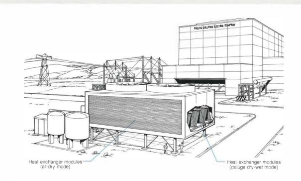
Figure 2 At the proposed demonstration facility to be installed on an existing 6-MW (e) turbine at PG&E's Kern plant, heat exchanger modules on the side of the cooling tower operate in the all-dry mode. Those visible in the cutaway at the end of the tower will demonstrate the deluge dry-wet option.
