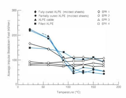
Figure 3 Average impulse breakdown strength as a function of temperature for filled and unfilled XLPE insulations and four EPR insulations.
