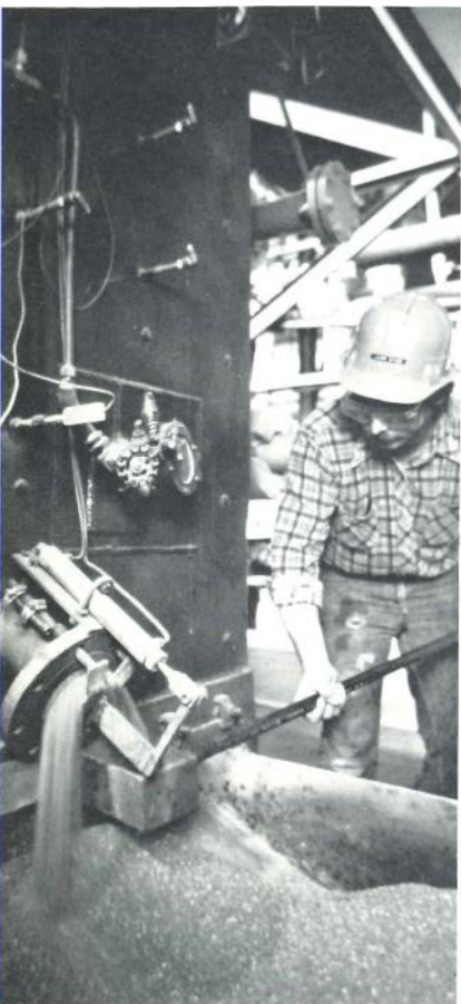
ability to recycle unburned coal and unreacted limestone back into the fluidized bed. The fully instrumented pilot has been providing researchers with a volume of useful data.
