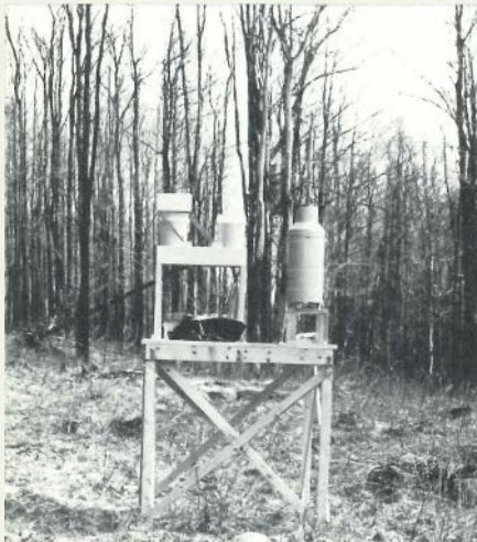
Figure 4 Atmospheric deposition and meteorological monitoring equipment in the Woods Lake watershed.
