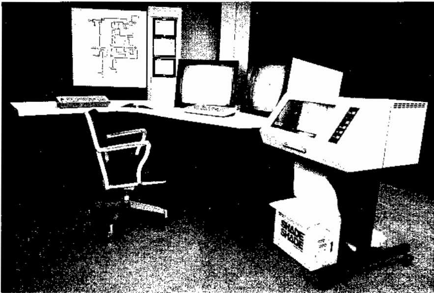
Figure 7 Dispatch operator console equipment that is being added to the EPRI hybrid computer. The combination will be evaluated as a dispatch operator training tool.
