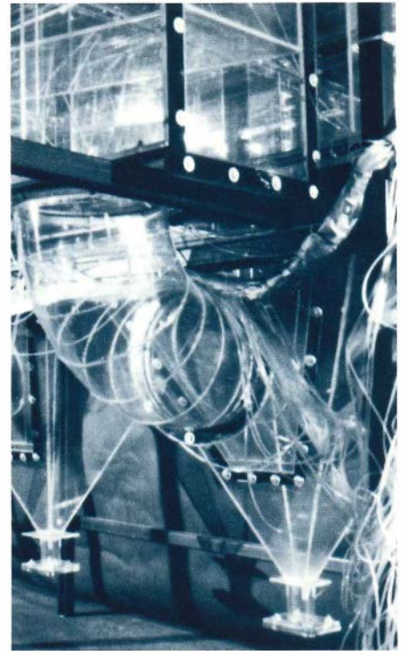
Transparent model (1/8 scale) of a baghouse used to study the flow distribution of gas and fly ash within the ductwork and compartments. Model is located in the research laboratory of Dynatech R/D Co., Cambridge, Massachusetts.
