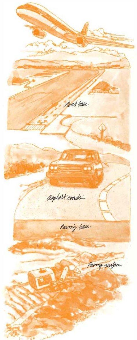
Roads, pavements, and parking lots are another category of applications for coal combustion by-products. Fly ash is used in road bases and asphalt roads; in fact, the runways and taxiways at the Newark, New Jersey, airport have fly ash in them. Bottom ash is used as aggregate in paving bases, and slag is used in paving bases and surfaces. Numerous states permit the use of by-products in highway construction.
