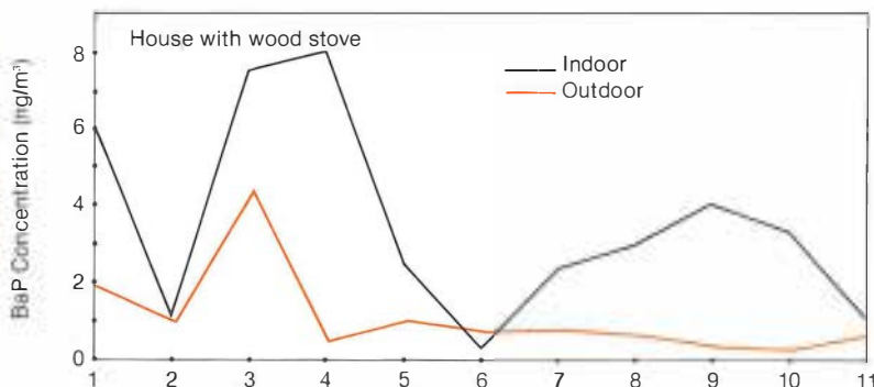
Patterns of household activity can have extreme effects on air quality in the home. In a residence with a wood stove (left), average levels of benzo-a-pyrene (BaP) were significantly higher than those outdoors except on days 2, 6, and 11, when the stove was not in use. In another case (right), a commercial oven cleaner caused levels of nonmethane hydrocarbons (NMHC) recorded in a kitchen to increase 16-fold in less than 90 minutes.
