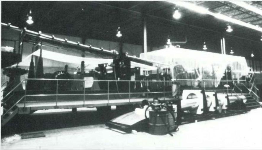
Figure 5 The UNIWEMA-450 can manufacture 230-kV and 345-kV cable in 100-m sections. Shown here is the machine forming the 390-mm enclosure as the flexible conductor is placed inside, with the spacer insulators attached. Lengths of more than 100 m could be made continuously; however, reel sizes would be prohibitively large and nearly impossible to ship by truck or rail.
