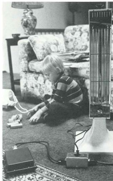
The Electric ARM (lower left) collects electricity use information on household appliances, such as this portable heater. These data can help utilities develop effective conservation and load management programs and assist in preparing load forecasts.
