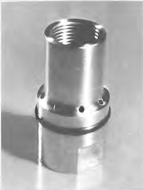
Figure 1 A five-orifice, sapphire-jeweled nozzle for cutting concrete.
