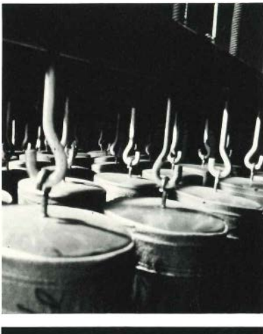
Fabric filter research is carried out at one of the seven independent pilot plants at the Arapahoe Emissions Control and Test Facility.
