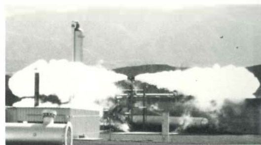
The PWR safety and relief valve test program satisfactorily demonstrated component operability under a range of full-scale conditions.
