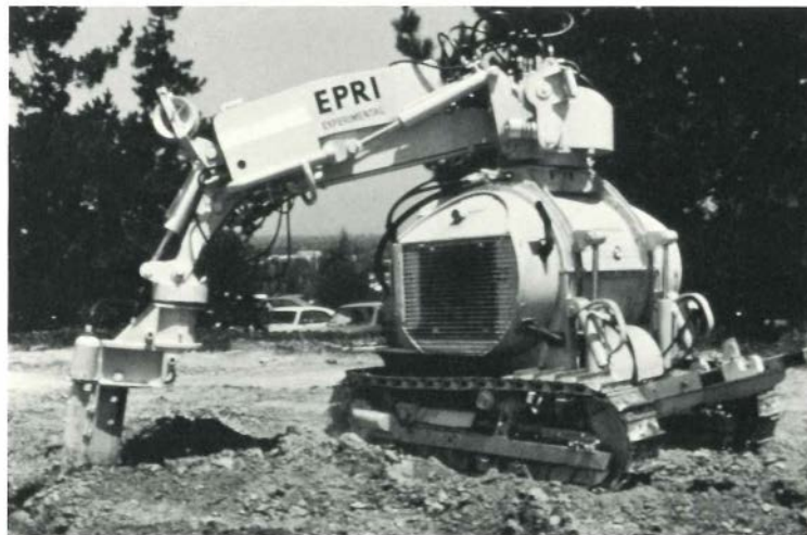
An advanced cable plow called the Scorpion can smoothly install underground distribution cable without trenching and backfilling.
