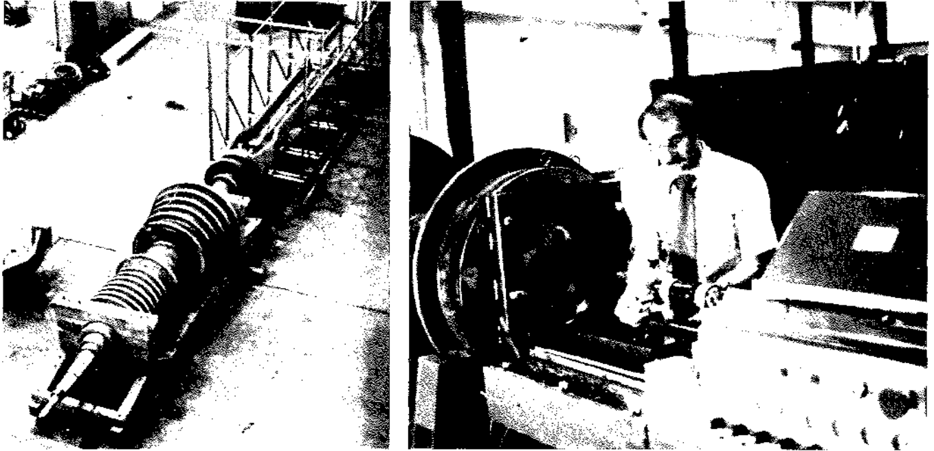
Figure 3 The NDE Center has completed an evaluation of an advanced inspection system for steam turbine rotors owned by American Electric Power Co., Inc. This system, called TREES (left), was compared with conventional technology represented by the BUCS system (right). The results, which show superior performance by TREES, are contained in NP-2640.
