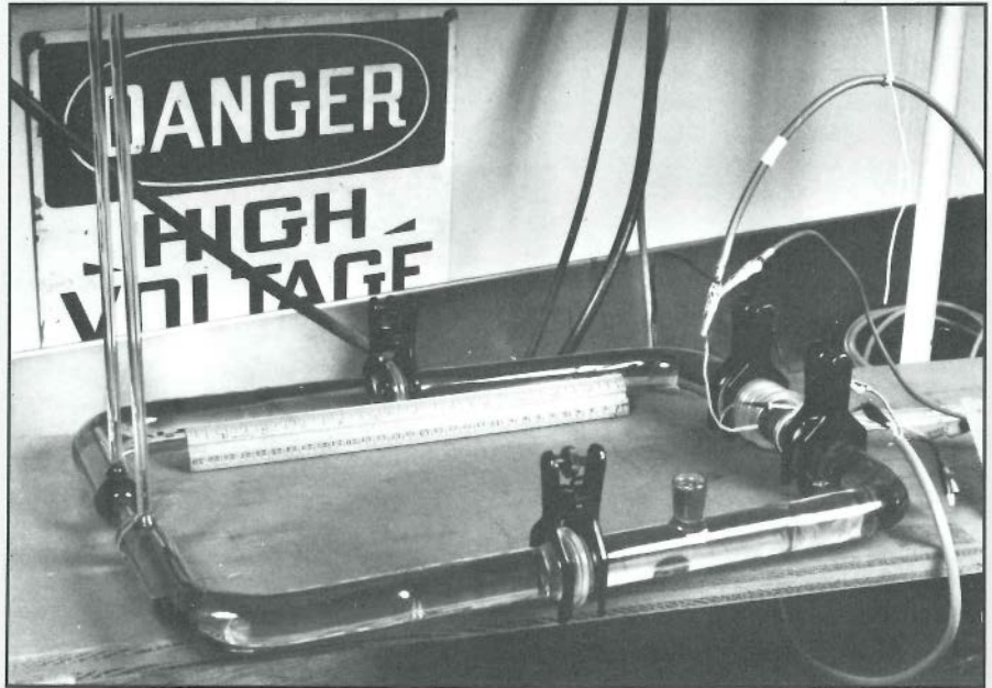
Figure 1 This bench-top apparatus was used in testing an electrohydrodynamic pump (which is contained in the section of glass tubing in the foreground). EHD pumping is being explored as a means of cooling distribution transformers.
