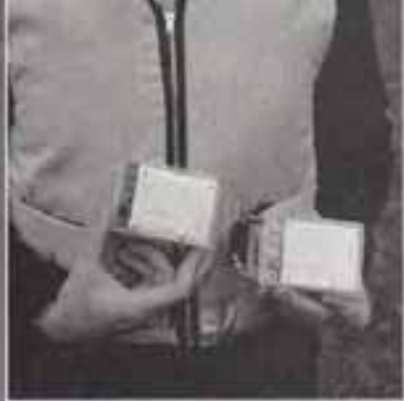
Specialty designed vests measure the cumulative exposure to various field strengths from high-voltage power lines as a farmer goes about his daily activities. An electrically conductive cloth overlay on the vest is attached to monitoring instrumentation.
