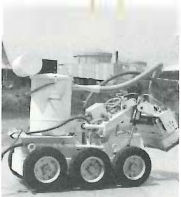
Remote scabbler (decontamination)
