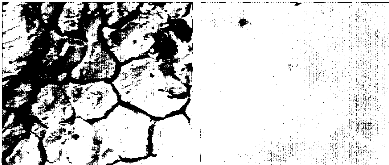
Figure 1 Scanning electron microscopy shows the topography of pipe interior surfaces before and after electropolishing: (left) the as-received surface, (right) after polishing for 24 minutes. Both micrographs have been magnified 500 times.
