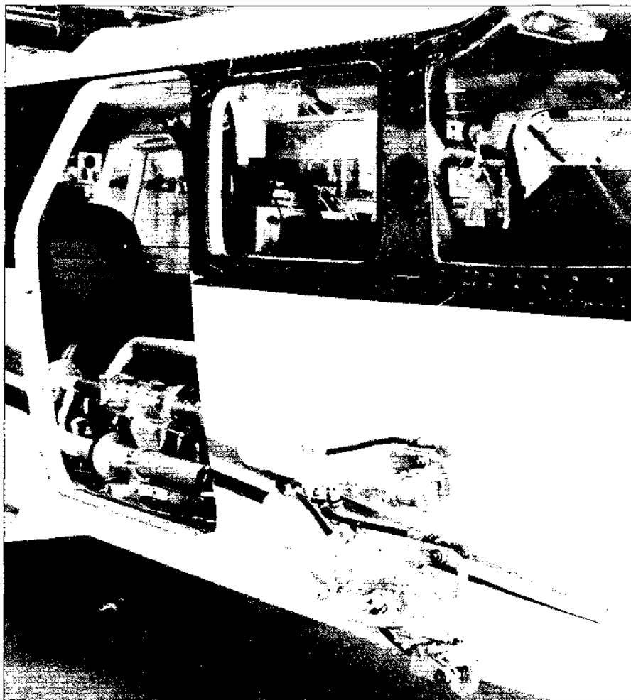
Figure 1 Cloud sampling devices on board an aircraft (Brookhaven National Laboratory). On the outer and inner sides of the fuselage, cloud water is sampled and separated from the interstitial aerosol with the CERL device; the aerosol is sampled and analyzed inside the cabin. Cloud water is collected through the top of the fuselage on slotted Teflon rods (developed at the State University of New York at Albany) and is saved for laboratory analysis.
