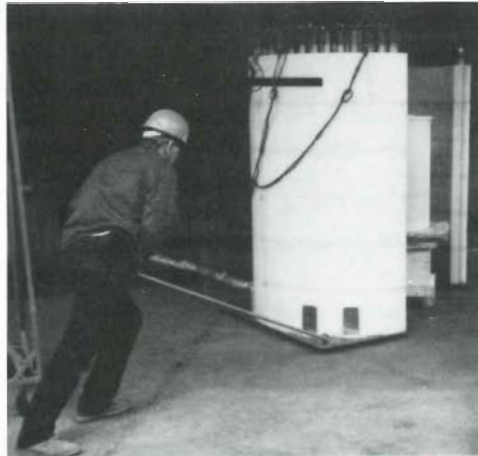
Closing detector assembly around radwaste drum.
