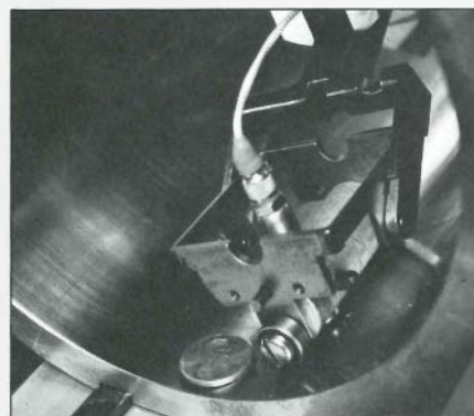
Figure 2 This new eddy-current sensor for turbine generator rotor bore surfaces promises improved flaw size sensitivity, greater repeatability, and reduced inspection time relative to conventional magnetic particle testing.
