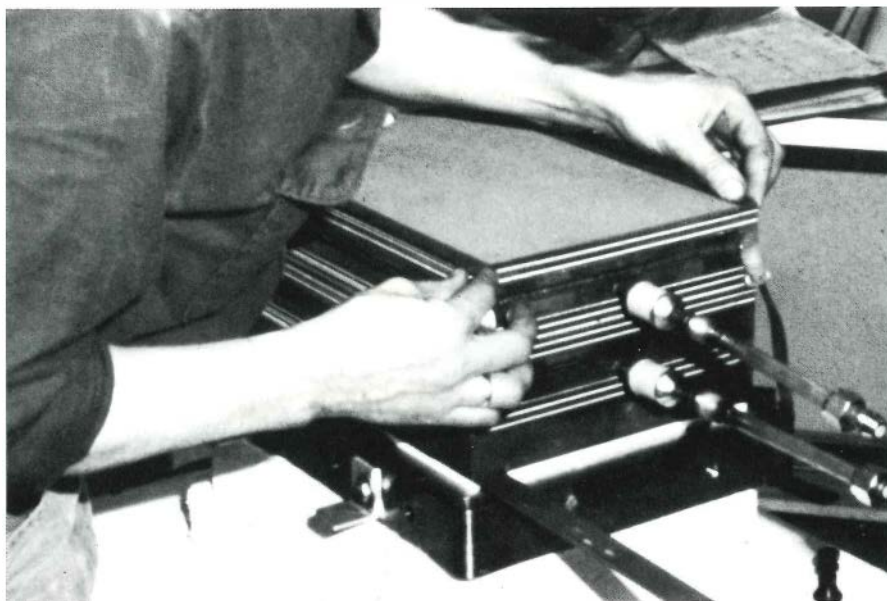
Figure 1 A prototype of the internal-reforming natural gas molten carbonate fuel cell, which has 10 cells and is about 1 ft 2 in size.
