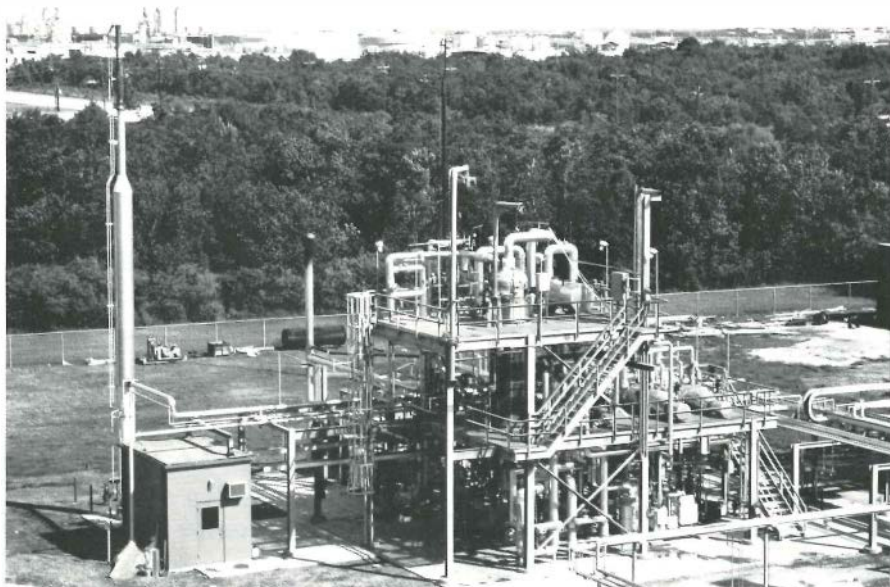
Figure 2 Full-scale 1.25-MW reformer module and supporting test facility installed near Houston, Texas. Natural gas and steam are catalytically converted into a hydrogen gas, the majority of which is flared to the atmosphere during a test. The EPRI test facility will be available to interested companies for special tests in 1988.
