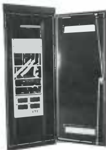
Yard data acquisition unit
