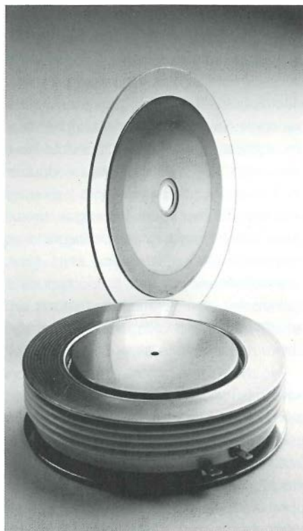
Figure 1 In high-power applications, standard thyristor packages (foreground) must contain metallic contact plates to disperse silicon-wafer-generated heat. By replacing the large contact plates with silicon, GE can produce a lighter package (background) with improved thermal performance for a quarter of the cost.
